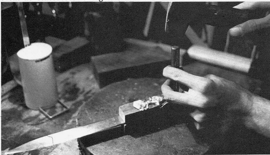
After pouring, the excess is hammered away leaving a firm, tight handle.
